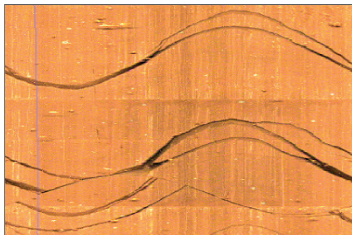
Left image: Partial picks (blue) show the continuation of the full sinusoid (dotted blue line) and allow picking of multiple visible segments (solid blue). Right image: Borehole wall image before picking.
