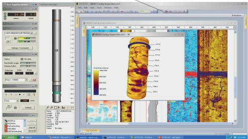
In this example, the operator is able to monitor the realtime scrolling log, view any or all other logs while monitoring all the log outputs, including depth. Optionally raw sensor data may be displayed. Comparison with main & repeat section, scrolling and adding annotations while data acquisition continues.
