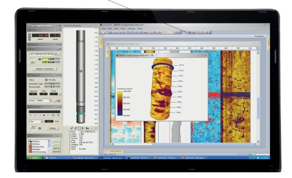
In this example, the operator is able to monitor the realtime scrolling log, view any or all other logs while monitoring all the log outputs, including depth. Optionally raw sensor data may be displayed. Comparison with main & repeat section, scrolling and adding annotations while data acquisition continues.
